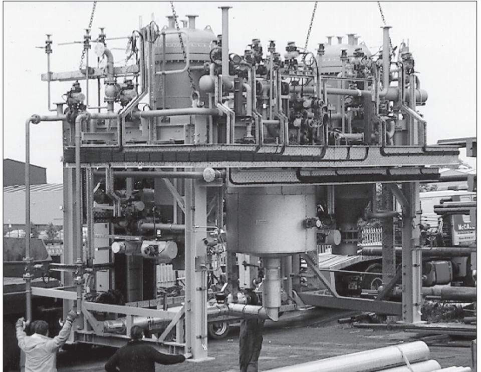
Figure 2: The photo shows the skid mounted FUNDABAC® filtration system during delivery to BP Oil Grangemouth refinery (Scotland). The two R-13 m2 filters are designed for simultaneous purification of two 73 m3/h lean DEA streams. Besides the two filter vessels, the insulated precoat tank, discharge valves and the control cabinet can be identified.
