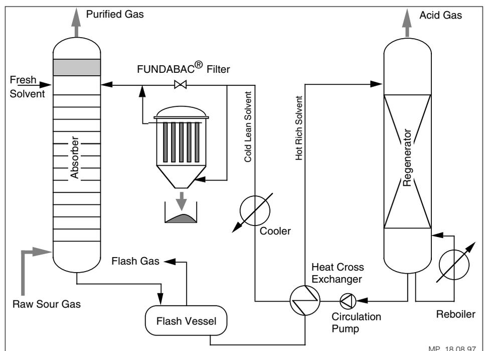
Figure 1: Basic configuration for a gas sweetening process utilizing a FUNDABAC® filter for removal of fine solid particles from the circuit.
